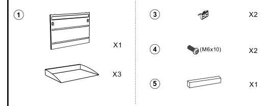
Place the sliding nuts (3) approximately 300 mm apart. Push them into the toolbar T-slot, then turn to make the spring face away from you.
