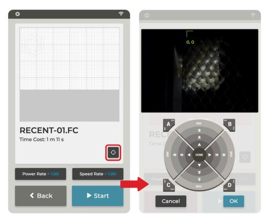
The origin point may be manually set before processing, and the power rate and speed rate can be set at any time during the process.
