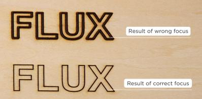
Thicker object: When the object is thicker or when the rotary add-on is used, the side of the object may be captured by the camera, and only the objects on the plane of focus can be stitched together, and the picture out of focus and inaccurate stitching caused by the height difference is normal. Be sure to focus on the surface of the engraving material and the highest point of the engraving material when using the rotary add-on.
