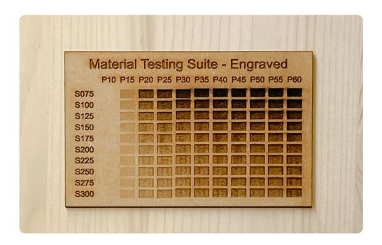
Use of the engraving or cutting sample file is not recommended with thin material (thickness less than 0.5 mm) due to the potential for excessive burning resulting in oversized engraving or cutting openings; begin manual testing of such materials with high speed and low power (e.g., P:15, S:300).
