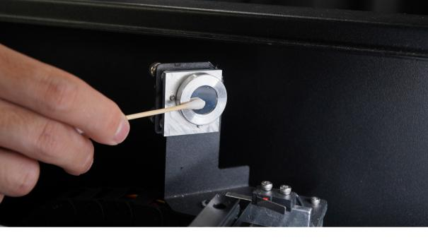
**2. Clean the second reflective mirror :** The second reflective mirror is located on the left Y-axis guiding rod facing the chassis.
