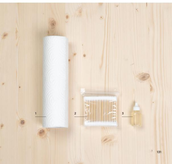
**1. Cleaning :** Use paper towel or tissue paper to wipe the oil and dust on the Y-axis guiding rods, X-axis linear rail and 4 lead screws.
