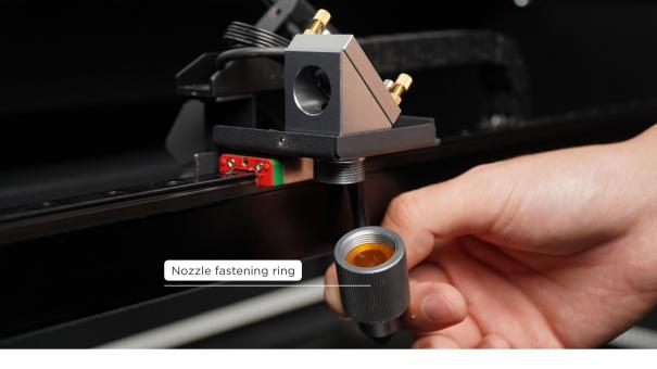
c. Unscrew the nozzle fastening ring clockwise > Remove the laser head, and please avoid the focus lens from being popped out >
