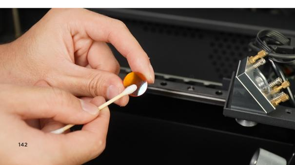
5. Put the focus lens back: The lens has an orientation, the convex side faces up, the flat side faces down.
