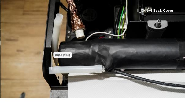
c. Insert the supplied water pipe and plug it into the water inlet of the laser tube to avoid to water leakage >
