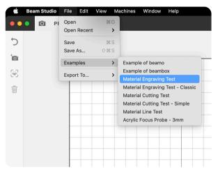
Try different combinations of speed (S: Speed) and power (P: Power) to find appropriate parameters for materials you have not worked with before. Sample test files can be imported through "Menu > File > Samples > Material Engraving Test. Test files are available for both engraving and cutting.
