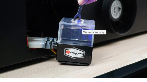
11. Tighten the water pump cap and the water pump cover back: Use the double head wrench to tighten the water pump cap back > Place the water pump in its original place > Tighten the 4 screws of water pump cover back with the Torx screwdriver.
