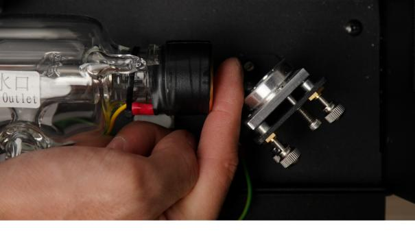
**6. Fix the laser tube holders :** Make sure the distance between the laser tube and the first reflective mirror is around 15mm (One finger's distance)
