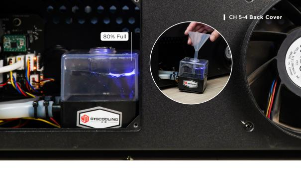
**9. Water Filling:** Open the cap of the pump with double head wrench > Put in the funnel > Pour the water in > Go to "Maintain Mode" and wait until it finishes homing > Press the "Pump" button to turn the water pump > When water tank's water decreases, pour in more eater until the tank is 80% full.
