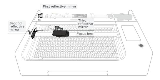
There are 3 reflective mirrors and 1 focus lens that need to be cleaned in HEXA, and their positions are shown in the picture.
