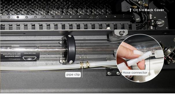
c. At Low-voltage side. put the clip on the shorter hose > Remove the plug > Insert the joint on both hoses > Move both clips closer to each other to prevent leakage.
