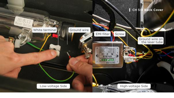
b. Disconnect the laser tube wires: Press the white terminal and pull out the ground wire > c. Remove the ground wire on the high-voltage side: Use the 2.5mm Allen Key to loosen the screws in the EMI filter. Put out the ground wire connected to the laser tube.
