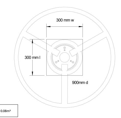
Minimum Concrete Specification: C16/20 (2900 N/mm² (20 N/mm²) min. compressive strength) Recommended Mix: 1 part cement/ 2 part sand/ 4 part stone.
