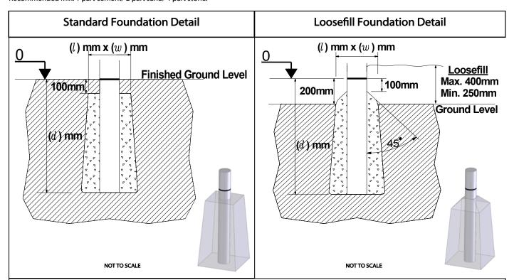
NOTE: All holes must taper out from hole width at top of hole (as shown) to give maximum stability. In loose or sandy ground all hole width dimensions should be increase by approximately 50%.
