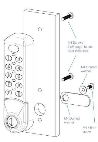
HOLES A, B & C DIAMETER 4.5 / 5.0mm HOLE D DIAMETER 16.0 / 16.5mm ALWAYS USE FIXING HOLE A USE EITHER OR BOTH OF HOLES B & C Recommended screw fixing torque 0.8Nm
