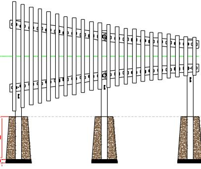
Compact base of hole with 50mm of aggregate. Lower ground Fix posts attached to instrument into hole (check instrument straight and level, and at correct height before filling with concrete) Foundations should not present a hazard. These foundations are recommended as a guide, for more information on foundation details for various surface see Part 7 of BS EN 1176.
