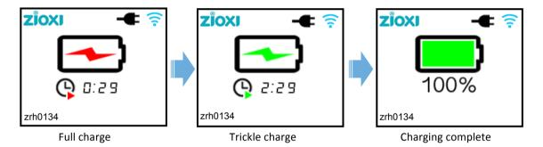
The length of time required for a full charge from a fully depleted battery will vary depending on the powerHub capacity but will typically be 12 to 16 hours. Once the powerHub has entered Trickle charge mode it is almost fully re-charged so can be used if required.
