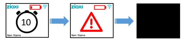
If the powerHub is left for a further period of time without re-charging then to protect it's batteries it will automatically turn off power to the powerHub sockets, display a red warning
