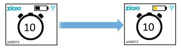
Once the battery gauge symbol changes from Black to Amber it is advisable to recharge the powerHub. Once the battery gauge changes to a single Red bar then the powerHub should be re-charged immediately.
