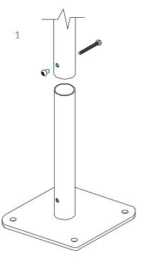
Locate the Surface fix Plate into the leg of the instrument.
